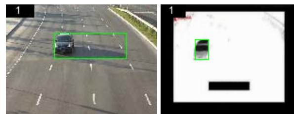
Fig. 11. Vehicle flow recognition at afternoon
