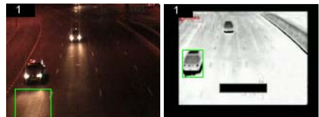
Fig. 10. Vehicle flow recognition at night
