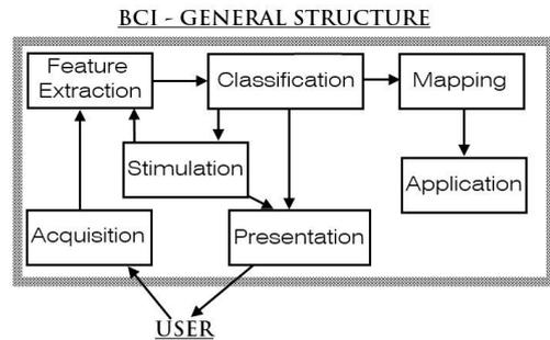
Fig. 2. General structure of a typical BCI system [8].
