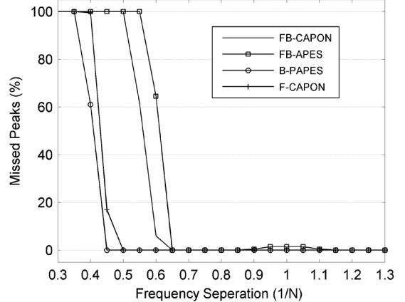
**Fig. 1.** Frequency resolution for filter length  $M=32$  and  $\text{SNR}=20$  dB in the case of two spectral lines
