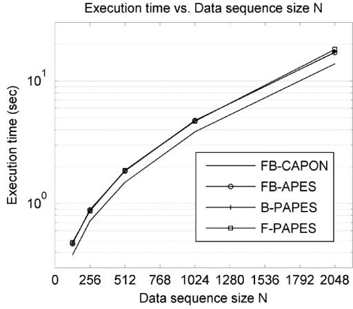
**Fig. 5.** Execution time for filter length  $M=N/2$  and SNR=14 dB in the case of random 1-D data sequences
