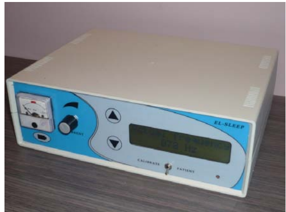
Fig. 7. Device for Cranial Electro Stimulation
