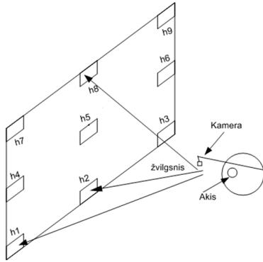
Fig. 4. Calibration points displayed on the monitor screen
