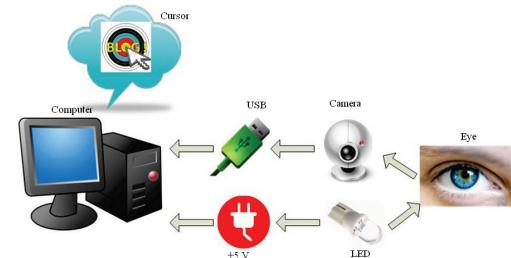
**Fig. 3.** The functional diagram of the system
