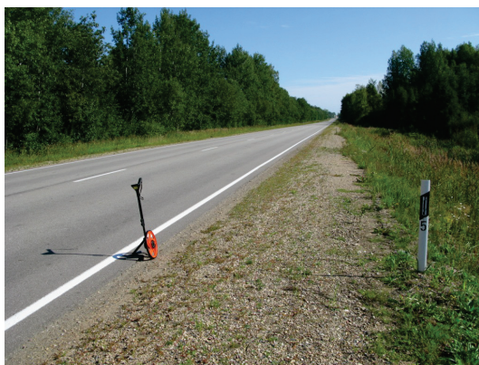
Fig. 3. Distance measurement by wheel between guide-posts on the road
