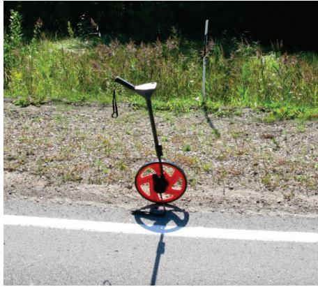
Fig. 2. Distance measuring wheel system
