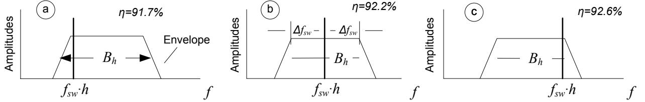
**Fig. 2.** Transformation of the harmonic  $h$  of the switching frequency  $f_{sw}$  into the appropriate band  $B_h$  in a consequence of FM of  $f_{sw}$ : b – for symmetrical FM; a, c – for asymmetrical ones
