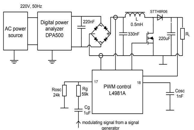
**Fig. 3.** Simplified schematic diagram of the experimental setup
