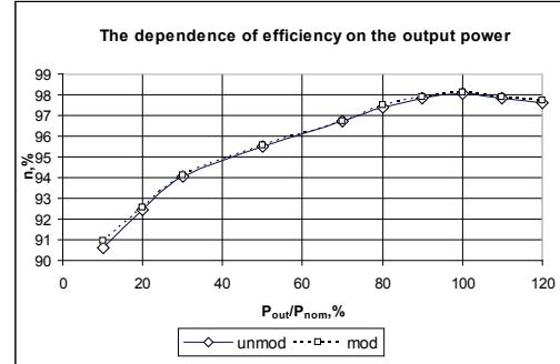
Fig. 5. The dependence of efficiency of PFC on the output power
