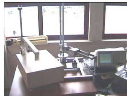
Fig. 3. A photograph showing the cartesian and cylindrical robot manipulators
