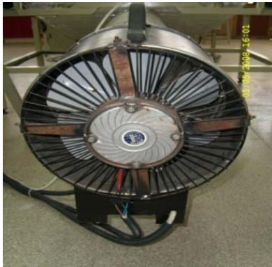
Fig. 4. Fan / heater used in the rotary drum dryer
