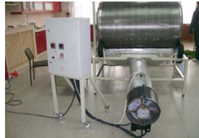
Fig. 1. General profile of a rotary drum dryer
