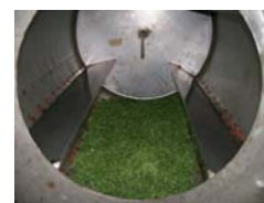
Fig. 2. Wings in the drum
