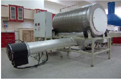
Fig. 3. Rotary drum dryer profile
