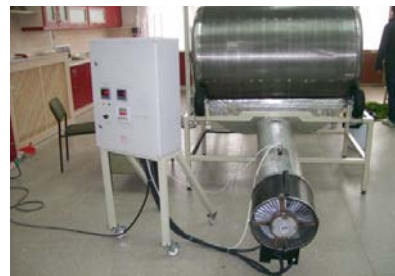
Fig. 1. General profile of a rotary drum dryer
