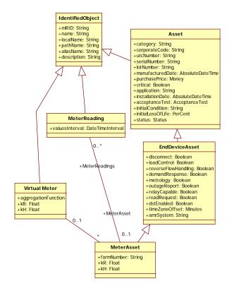
Fig. 2. CIM model with Virtual Meter
