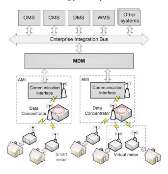
Fig. 1. Open Smart Metering architecture
