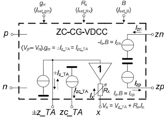
Fig. 1. Symbol and behavioral model of the ZC-CG-VDCC.
