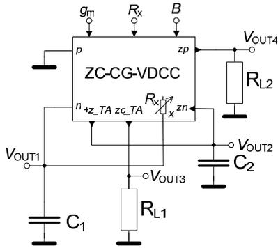
Fig. 2. ZC-CG-VDCC based second-order simple multiphase oscillator.
