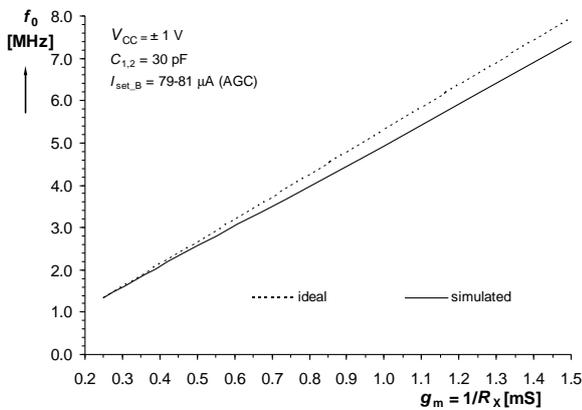
Fig. 9. Dependence of oscillation frequency on  $g_m = 1/R_x$ .
