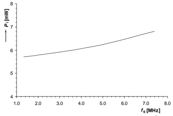
Fig. 13. Dependence of power consumption on oscillation frequency.
