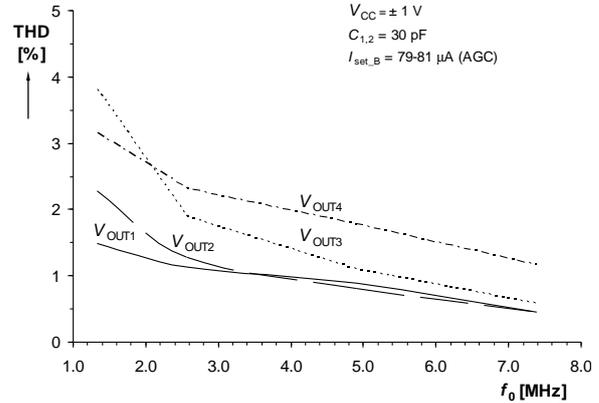
Fig. 12. Dependences of THD on oscillation frequency.
