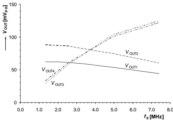
Fig. 11. Dependences of output levels on oscillation frequency.
