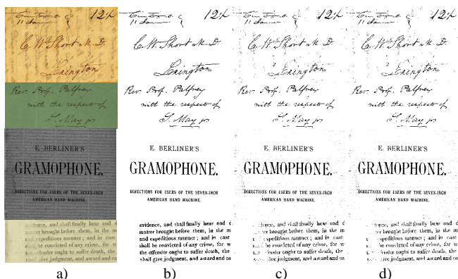
Fig. 9. The binarization results using the proposed method for chosen images from DICOM2011 dataset: original images (a), “ground truth” (b), results of Otsu binarization (c) and using the proposed method (d).
