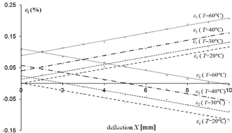
Fig. 6. The relative resistance increments  $\varepsilon_1, \varepsilon_2$  in the function of the beam  $X$  deflection while temperature  $T$  is changing.
