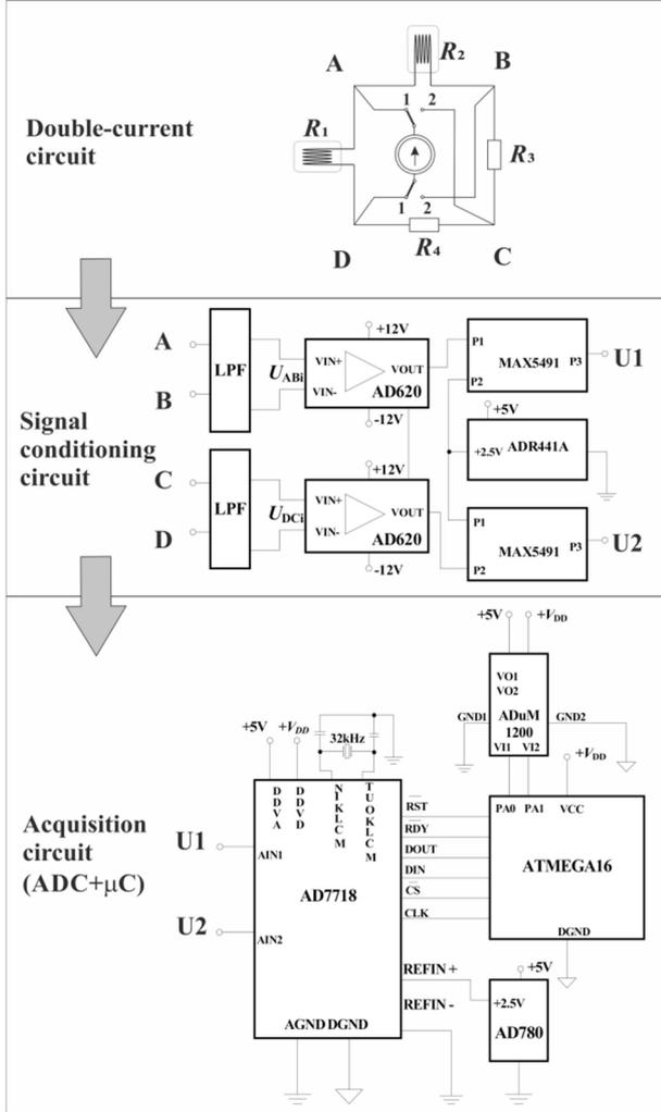
Fig. 2. Double current bridge for measurement of two variables [10].
