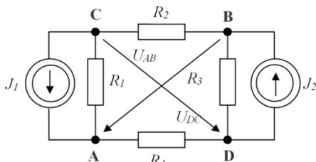
Fig. 3. Double current bridge (2J) – theoretical circuit [7].
