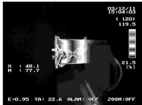
Fig. 8. Temperature distribution on the beam and a measurement in the strain gauge localization (heater was hidden in order to better illustrate temperature distribution around a strain gauge).
