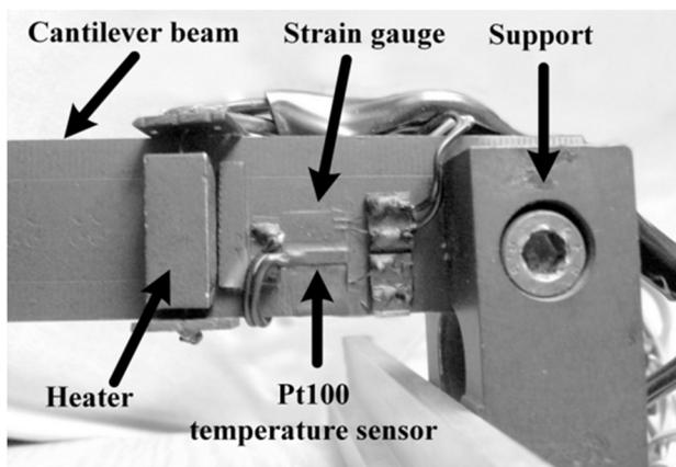
Fig. 7. Localization of heater, RTD sensor and strain gauge.
