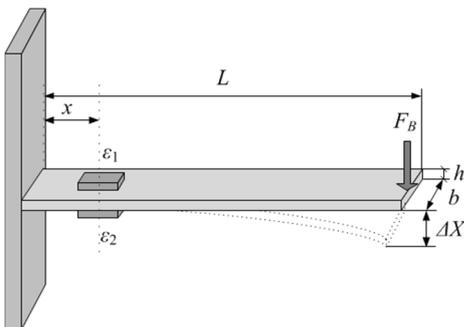
Fig. 4. Two metal strain gauges placed on the cantilever beam. The beam is bent by force  $F_B$  and heated in the same time.
