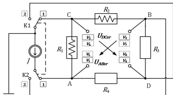
Fig. 1. Double current bridge (2x1J) as an input analog part of measurement system (J-current source,  $R_1$ ,  $R_2$  – sensors,  $R_3$ ,  $R_4$  – resistors, K1, K2 – electronic switches).
