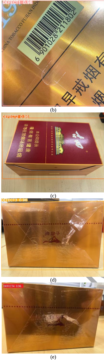
Fig. 6. Experimental detection precision: (a) Detection P = 0.97 for Good condition; (b) Detection P = 0.96 for Defect-1 condition; (c) Detection P = 0.96 for Defect-2 condition; (d) Detection P = 0.96 for Defect-3 condition; (e) Detection P = 0.97 for Defect-4 condition.
