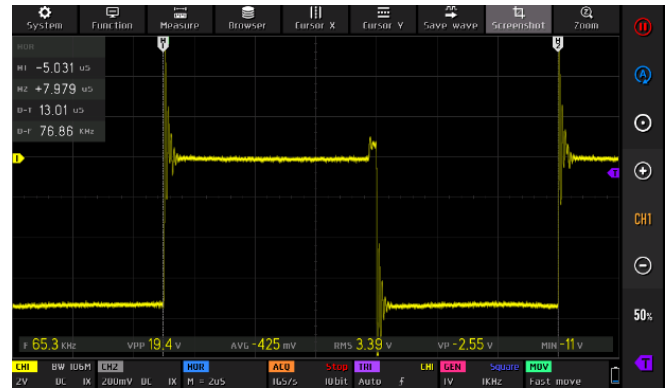
Fig. 9. DJI Mini 2 PWM switching frequency of ESC at 76.8 kHz at the period of H1-H2.
