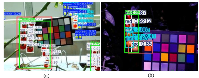
Fig. 10. Examples of harvesting decision results: (a) Multiple clusters mistakenly recognized as a single cluster; (b) Decision affected by an error in determining the lowest ripeness position of a cluster.
