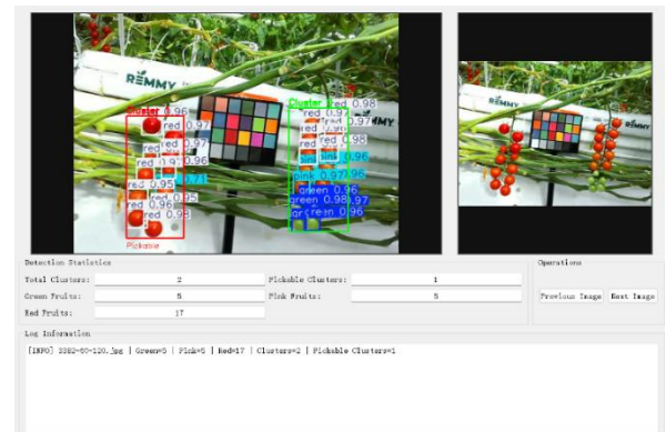
Fig. 9. Visualization of the tomato harvesting decision system. It provides the number of each fruit type, the total truss count, and the pickable truss count, intuitively showing the distribution of fruits and the status of each truss.
