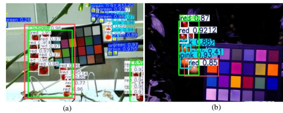
Fig. 10. Examples of harvesting decision results: (a) Multiple clusters mistakenly recognized as a single cluster; (b) Decision affected by an error in determining the lowest ripeness position of a cluster.
