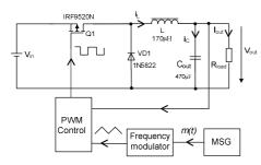
Fig. 1. Schematic of FM closed-loop buck converter used.
