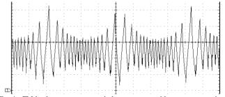
Fig. 4. FM buck converter power inductor current without core saturation effects. Parameters:  $f_{sw0}$ =100kHz;  $f_m$ =5kHz;  $\Delta f_{sw}$ =35kHz. (Scale: 50us/div; 100mA/div).
