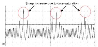
Fig. 5. FM buck converter power inductor current with core saturation effects. Parameters:  $f_{sw0}$ =100kHz;  $f_m$ =5kHz;  $\Delta f_{sw}$ =35kHz. (Scale: 50us/div; 400mA/div).
