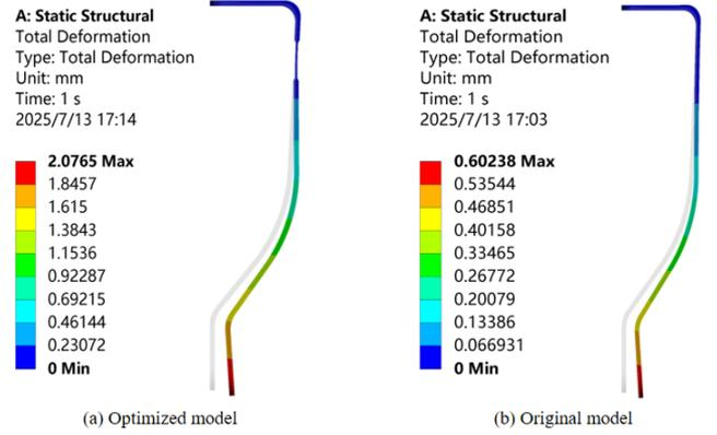
Fig. 5. Displacement distribution of the cantilever beam: (a) Optimised model; (b) Original model.
