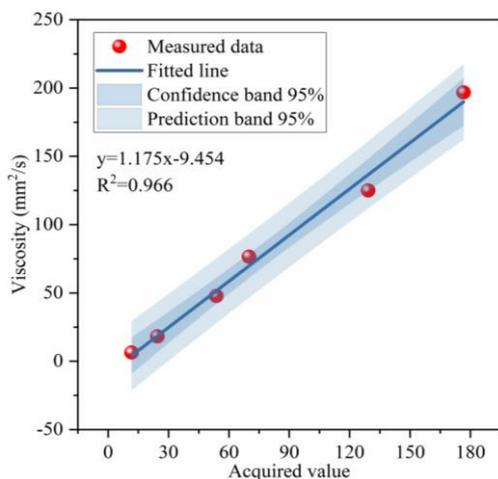
Fig. 8. Calibration curve between the acquired value and the standard kinematic viscosity.
