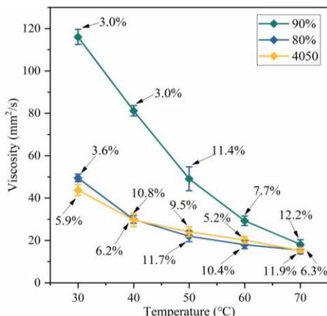
Fig. 11. Effect of temperature on viscosity for different samples.
