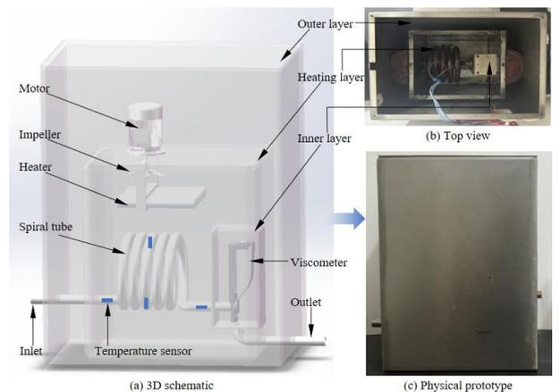
Fig. 1. Structural design of the viscosity measurement device: (a) 3D schematic; (b) Top view; (c) Physical prototype.
