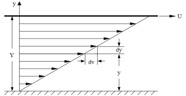
Fig. 4. Illustration of viscous behaviour in fluids.
