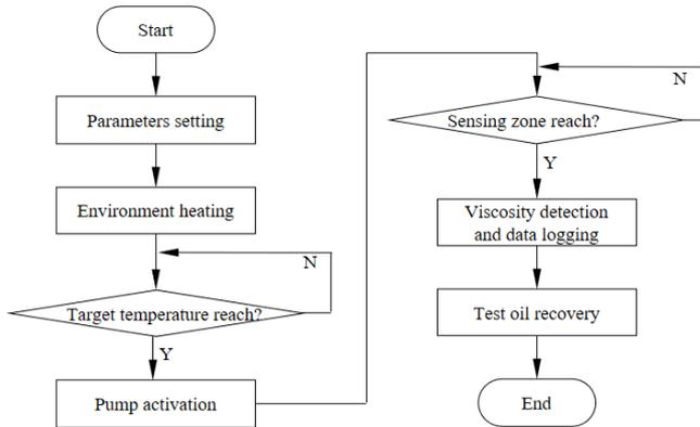
Fig. 2. Operational workflow of the viscosity measurement process.
