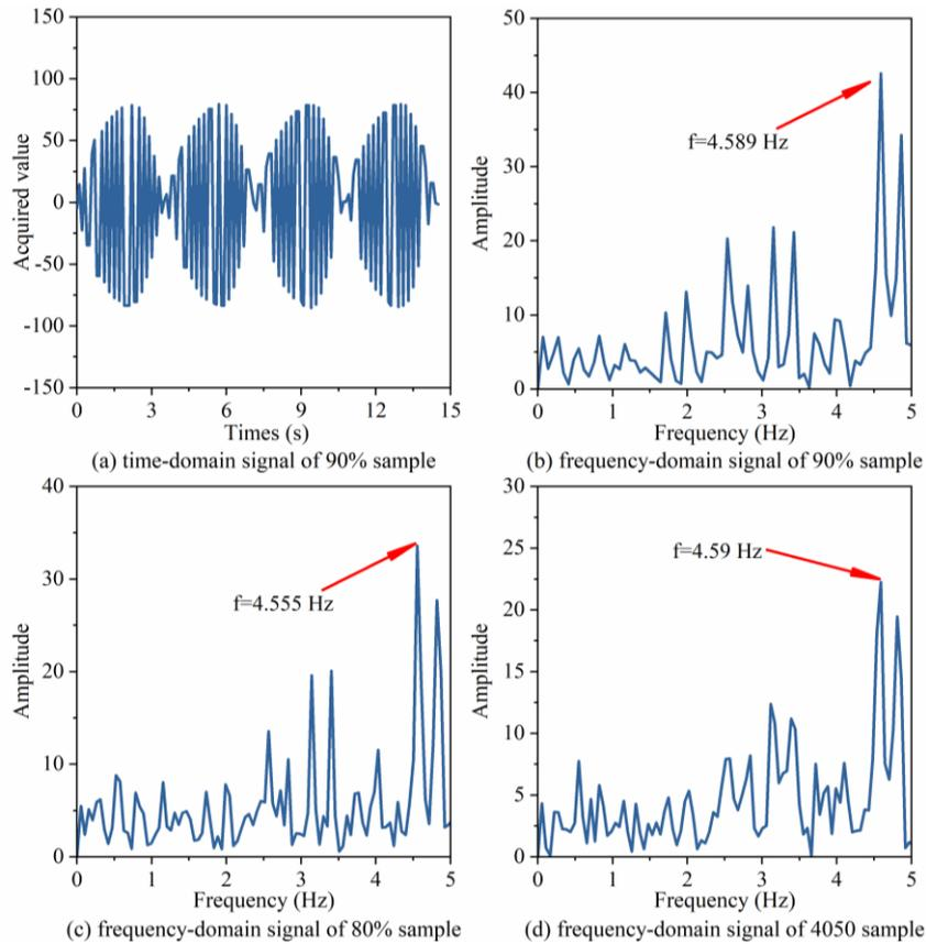
Fig. 10. Time- and frequency-domain analysis of viscosity signals: (a) Time-domain signal of 90 % sample; (b) Frequency-domain signal of 90 % sample; (c) Frequency-domain signal of 80 % sample; (d) Frequency-domain signal of 4050 sample.
