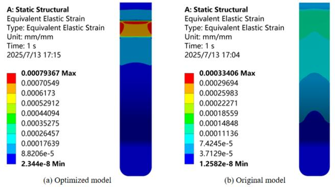
Fig. 6. Stress distribution of the cantilever beam: (a) Optimised model; (b) Original model.
