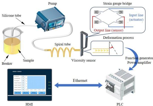
Fig. 3. Overall system architecture and signal flow.
