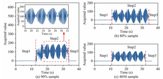
Fig. 9. Viscosity sensor signals for three test samples at 30 °C: (a) 90 % sample; (b) 80 % sample; (c) 4050 sample.
