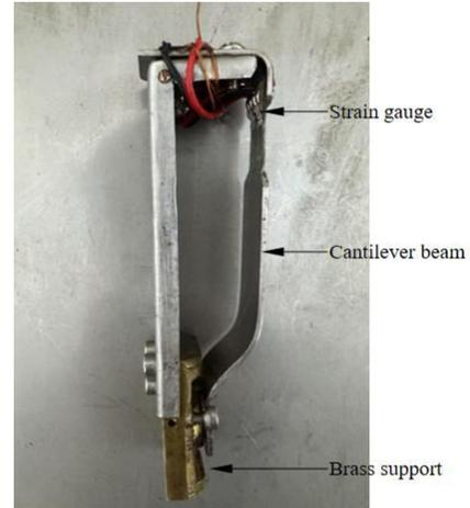
Fig. 7. Physical prototype of the optimised viscosity sensor.
