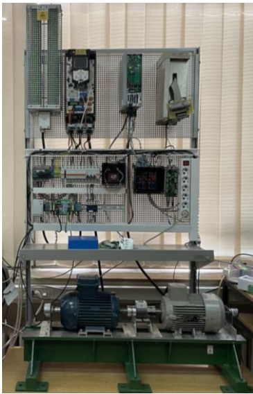
Fig. 7. Experimental setup used to measure the speed-time characteristics of the IM.
