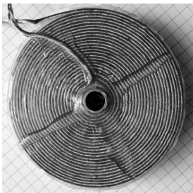
Fig. 3. Experimental flat coil with enameled copper wire (on left) and litz wire (on right).
