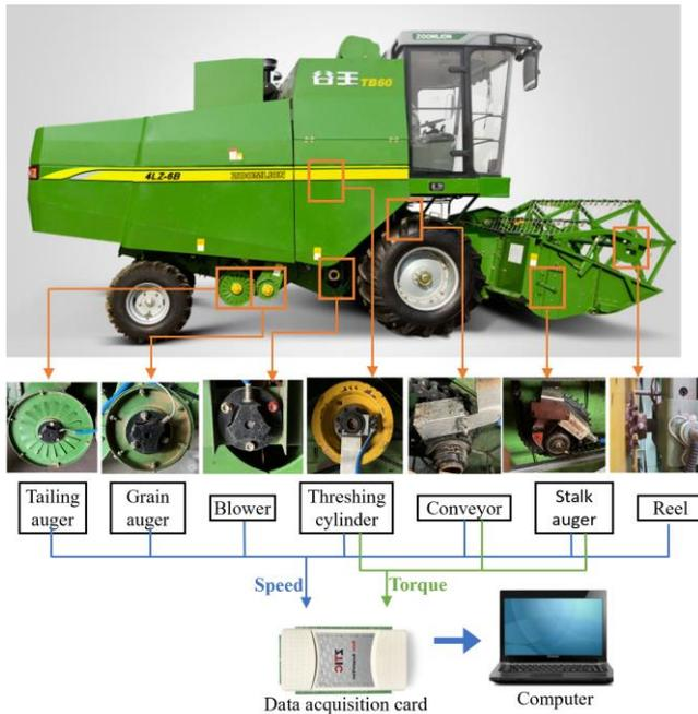
Fig. 2. Data acquisition system.
