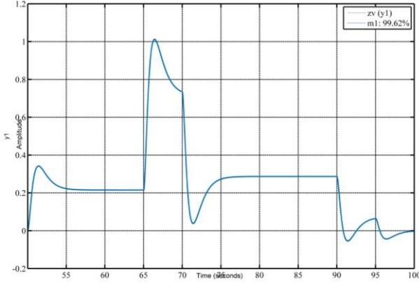
Fig. 9. Comparison of the simulated response of the multi-tank system ( $z_v$  signal) and the H-W model of the system ( $m_1$ ). Both the input and output nonlinearities of an H-W model have been represented using  $\varphi_{2ML}^{(\delta)}(t)$  function.
