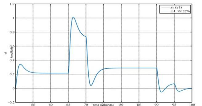
Fig. 8. Comparison of the simulated response of the multi-tank system ( $z_v$  signal) and the H-W model of the system ( $m_1$ ). The input and output nonlinearities of an H-W model have been represented using  $\varphi_{1ML}^{(\delta)}(t)$  and  $\varphi_{1ML}^{(\delta)-1}(t)$  functions.
