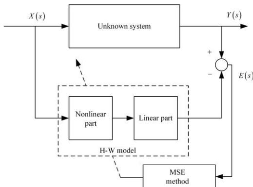
Fig. 6. Block scheme of system identification.
