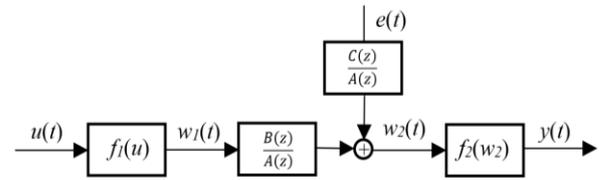
Fig. 3. H-W ARMAX system.
