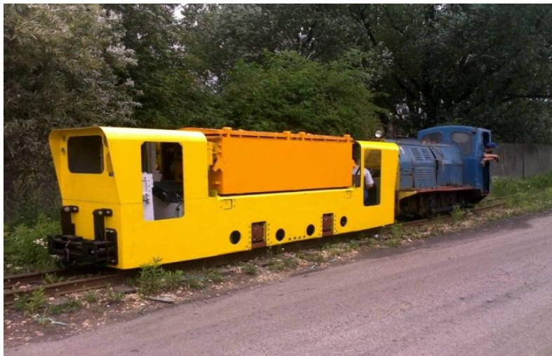
Fig. 8. Modernized Lea BM-12 locomotive with transportation load in a form of diesel locomotive [7].
