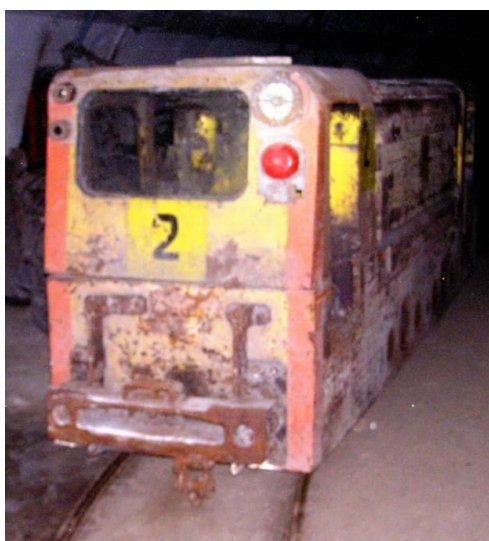
Fig. 1. Battery supplied mining locomotive Lea BM-12 [1].
