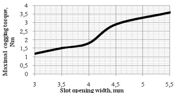
Fig. 5. Dependence of maximal cogging torque vs. slot opening width.
