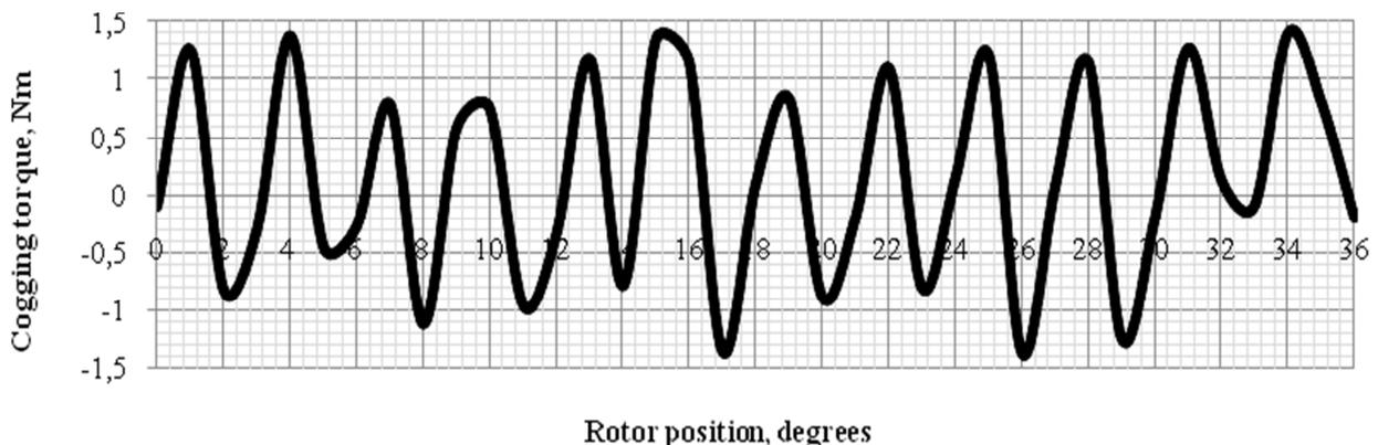
Fig. 4. Dependence of cogging torque vs. rotor angle.
