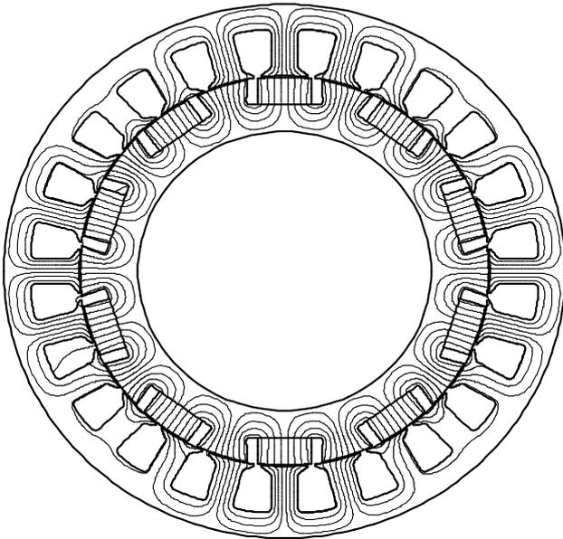
Fig. 3. The distribution of magnetic flux in machine cross-section
