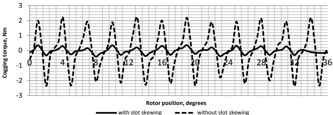
Fig. 8. Curves of change of the cogging torque at rotational rotor with stator slot skewing and without.
