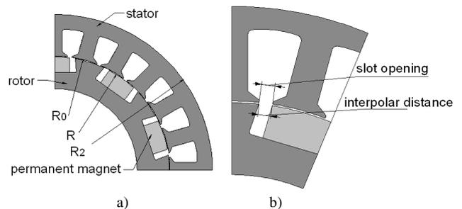
Fig. 1. Cross section of the PMSG.
