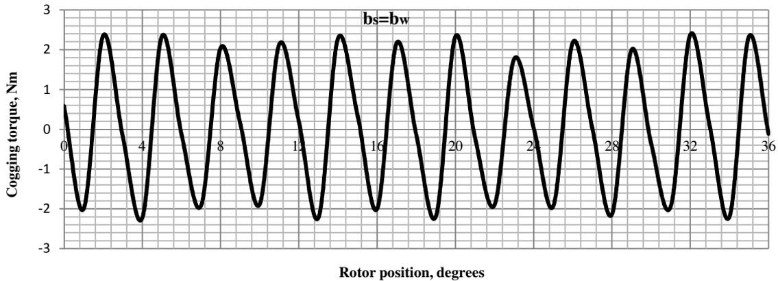
Fig. 6. Dependence of cogging torque on rotor angle.
