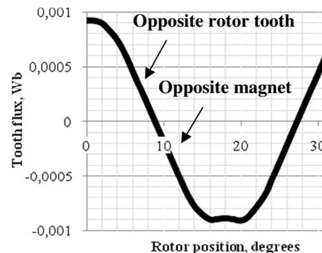
Fig. 2. Change of flux in stator tooth vs. rotor position.
