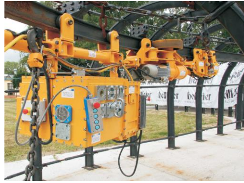
Fig. 1. General view of the installation of a selected suspended battery vehicle (PCA-1).
