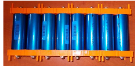
Fig. 2. Battery pack arranged of eight lithium-iron-phosphate (LiFePO 4 ) cells for testing.
