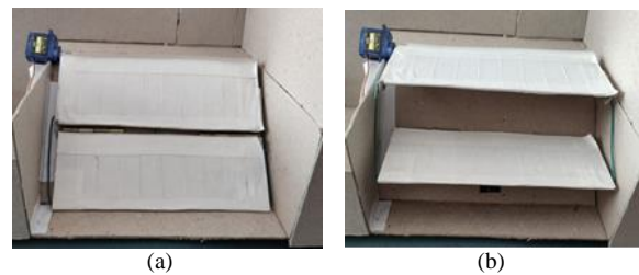
Fig. 7. The prototype of the barrier-free staircase: (a) ramp case, (b) stair case.
