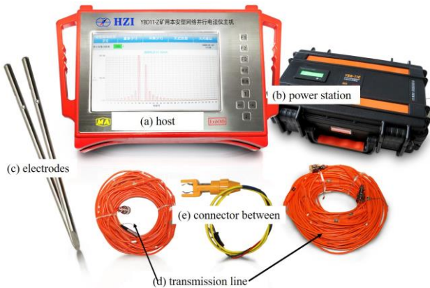
Fig. 4. Mine direct resistivity equipment: (a) host, (b) power station, (c) electrodes, and (d) transmission line. Problems of Forward and Inversion.
