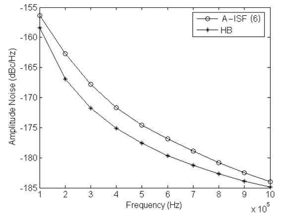
Fig. 10. Amplitude noises calculated by HB and (6) for 19-stage ring oscillator.
