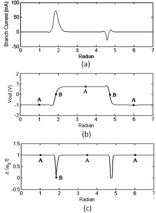
Fig. 6. (a) Branch current (b) output voltage (c) A-ISF (ring oscillator).
