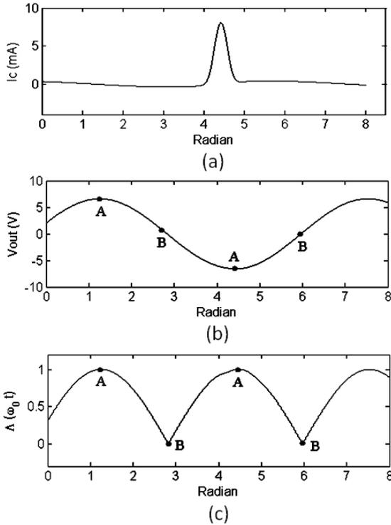
Fig. 4. (a) Transistor current (b) output voltage (c) A-ISF (Colpitts oscillator,  $R=10\text{k}\Omega$ ,  $L=200\text{nH}$ ,  $C_1=40\text{pF}$ ,  $C_2=200\text{pF}$ ,  $f=62\text{MHz}$ ).
