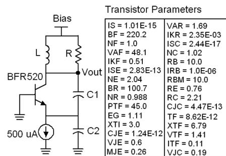
Fig. 3. The Colpitts oscillator.
