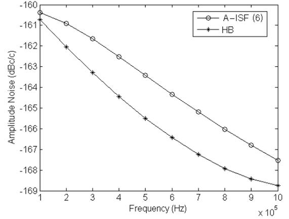
Fig. 9. Amplitude noises calculated by HB and (6) for Colpitts oscillator with  $R=10$ k $\Omega$ ,  $L=200$ nH,  $C_1=40$ pF,  $C_2=200$ pF.
