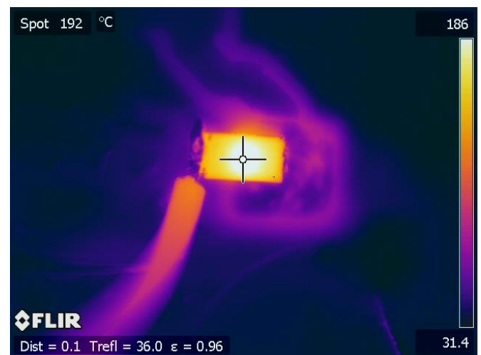
Fig. 9. The measured temperature for 500 [mA] forward current.
