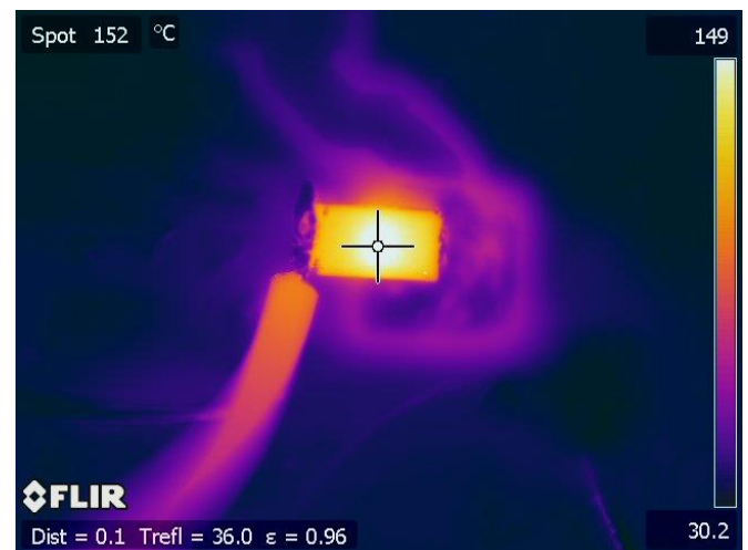
Fig. 8. The measured temperature for 410 [mA] forward current.
