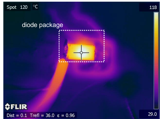
Fig. 7. The measured temperature for 300 [mA] forward current.
