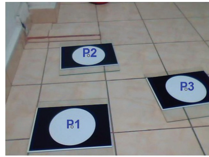
Fig. 5. Ground plane localization using three circles
