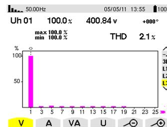
Fig. 7. Spectrum of the line voltage.
