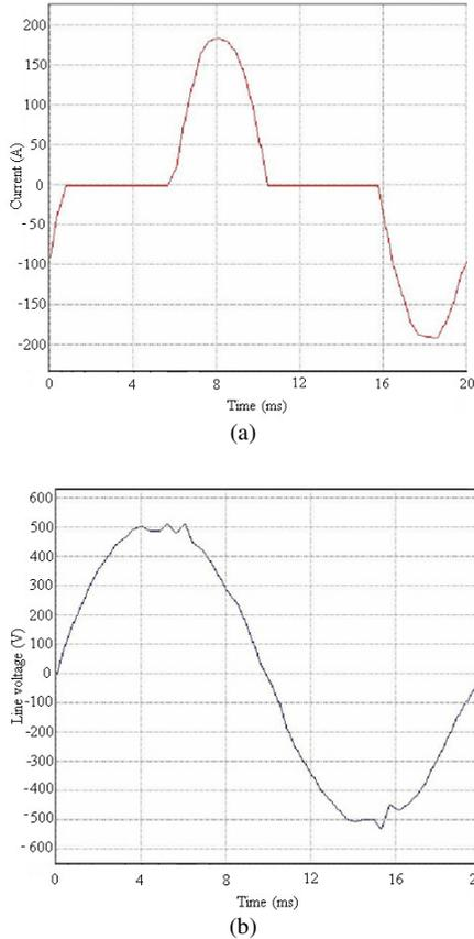
Fig. 4. Measured primary source current (a) and voltage (b) for an ESP power supply.
