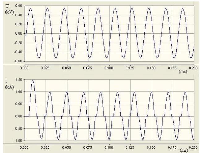
Fig. 11. Source voltage ( $V_{source}$ ), source current ( $I_{source}$ ), for power supply from Fig. 10,  $\alpha=90^\circ$  (THD=20.41%).
