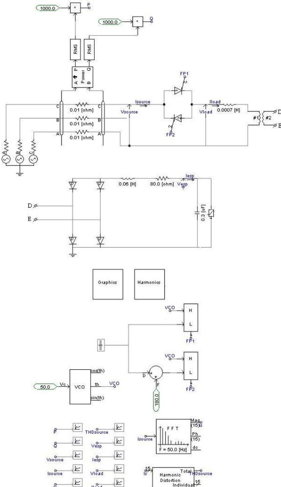
Fig. 10. Electrical installation of the ESP section using in simulations.
