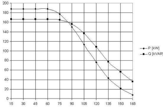
Fig.13. Effective active power (P) and effective reactive power (Q) depends on  $\alpha$ .
