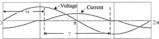
Fig. 2. Voltage and current through TCR.
