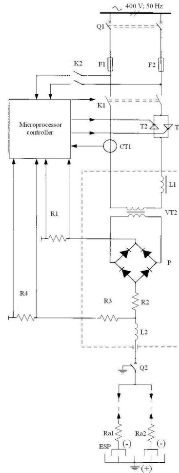
Fig. 3. Electrical power supply for a section.
