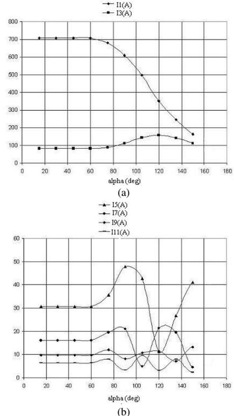
Fig. 12. Source current harmonic: a.  $I_1$  and  $I_3$ ; b.  $I_5$ ,  $I_7$ ,  $I_9$ , and  $I_{11}$  for  $\alpha = 15...165^\circ$ .
