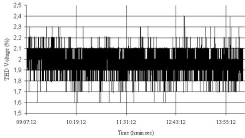
Fig. 9. THD line voltage of ESP power supply for a few hours operation.
