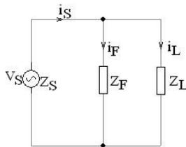
Fig. 14. Operation of passive filter.
