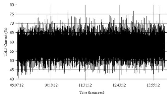
Fig. 8. THD current of ESP power supply for a few hours operation.
