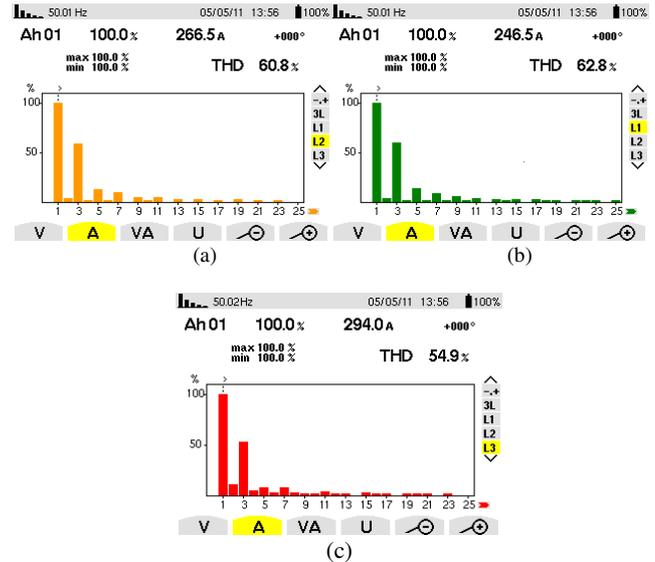
Fig. 6. Spectrum of current along one minute period of time.
