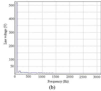
Fig. 5. Spectrum for primary source current (a) and spectrum for source voltage (b) for an ESP power supply.
