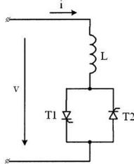
Fig. 1. Thyristor-controlled reactor (TCR) principle.
