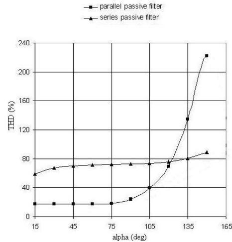
Fig. 16. THD current depends on firing angle  $\alpha$  with passive filters.
