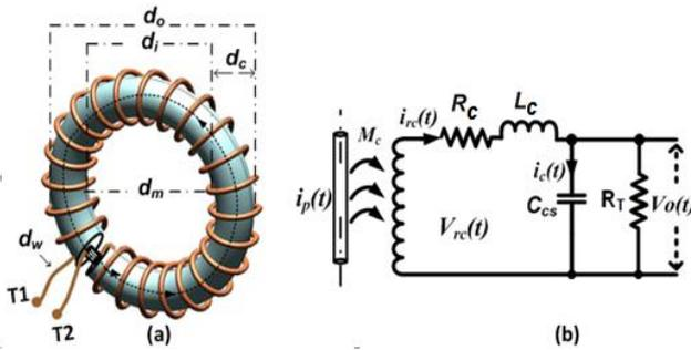
Fig. 1. Model of Rogowski coil. (a) Geometrical parameters model. (b) Lumped parameters model.
