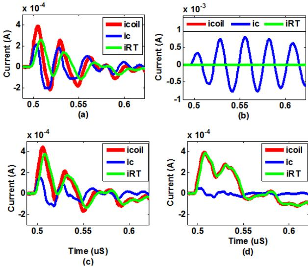
Fig. 7. Current  $i_{coil}$ ,  $i_c$  and  $i_{RT}$  through the components of  $L_c$ ,  $C_{cs}$  and  $R_T$  of Rogowski coil respectively for different value of  $R_T$ : (a)  $R_T = 1M\Omega > Z_c$ ; (b)  $R_T = Z_c$ ; (c)  $R_T = Z_c/2$ ; (d)  $R_T \leq Z_c/2$ .
