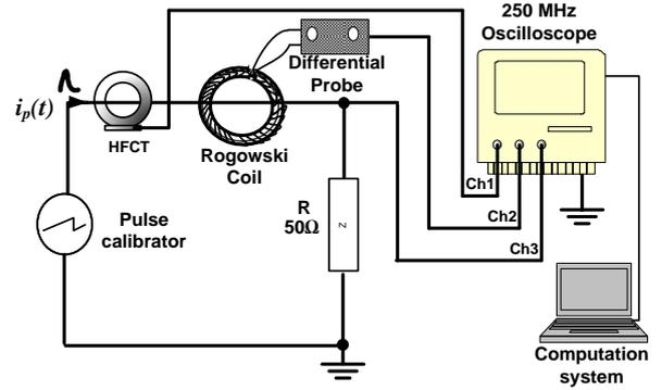
Fig. 2. Laboratory experimental setup for Rogowski coil measurements.
