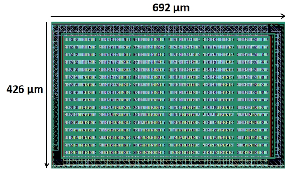
Fig. 1. A high voltage power MOSFET designed in a partial SOI process.
