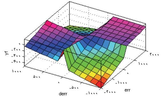
**Fig. 2.** Fuzzy rule emotional parameter in 3D input
