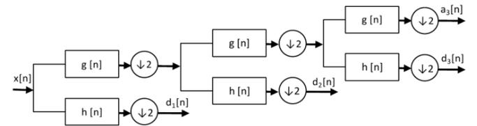
Fig. 2. Wavelet decomposition over 3 levels.
