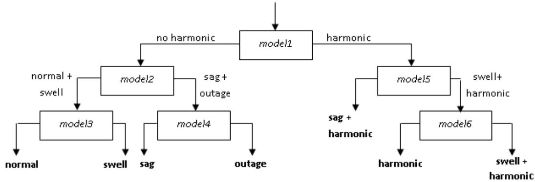
Fig. 4. Classification of the power disturbances using SVM decision tree.
