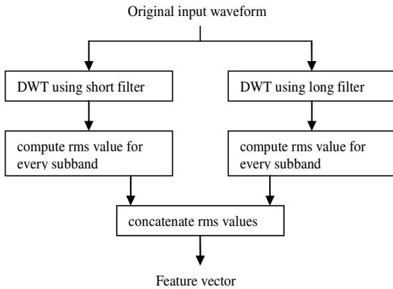
Fig. 1. Feature vector construction procedure.
