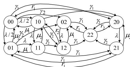
Fig. 2. Detailed Markov chains of an unreliable system with two channels, data packet losses and Poisson data packet arrival
