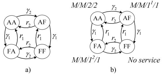
**Fig. 3.** Markov chains for the macro states of an unreliable system
