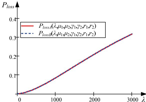
**Fig. 4.** Results of data packet transmission loss obtained by the means of detailed states Markov model –  $P_{lossA}$  and the macro states Markov model –  $P_{lossB}$  as a function of data packet arrival rate  $\lambda$ , when  $\mu_1=\mu_2=\mu=2000$  pack/s,  $\gamma_1=1/5000$  [hours $^{-1}$ ],  $\gamma_2=1/1000$  [hours $^{-1}$ ],  $r_1=r_2=1/24$ [hours $^{-1}$ ]
