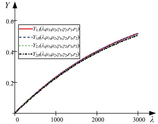
**Fig. 5.** Results of data packet transmission channels utilization obtained by the means of detailed states Markov model –  $Y_{1A}, Y_{2A}$ , and the macro states Markov model –  $Y_{1B}, Y_{2B}$  as a function of data packet arrival rate  $\lambda$ , when  $\mu_1=\mu_2=\mu=2000$  pack/s,  $\gamma_1=1/5000$  [hours $^{-1}$ ],  $\gamma_2=1/1000$  [hours $^{-1}$ ],  $r_1=r_2=1/24$ [hours $^{-1}$ ]
