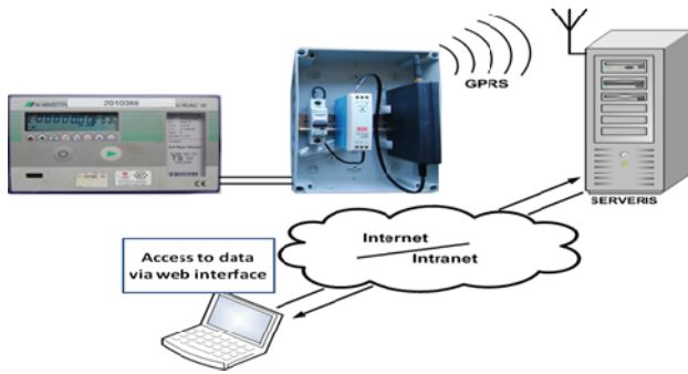
Fig. 3. A block scheme of technical solution for automatic metering data reading from energy meters
