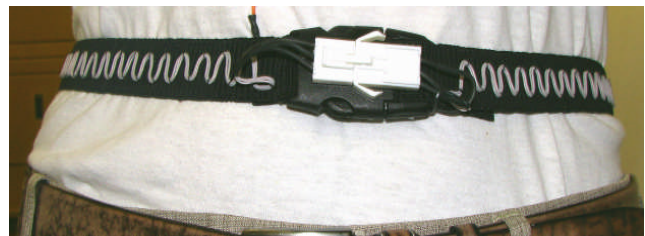
Fig. 1. The inductive strap of the respiration rate sensor
