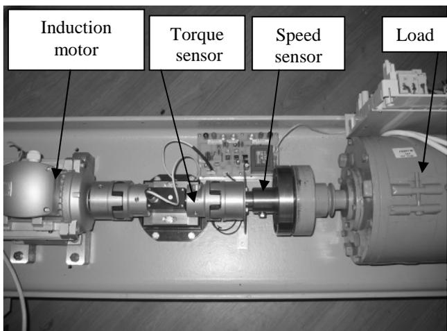
**Fig. 4.** The laboratory setup for experimental investigation
