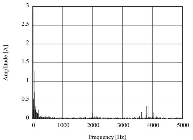
**Fig. 6.** Motor current spectrum at  $f_p = 40$  Hz
