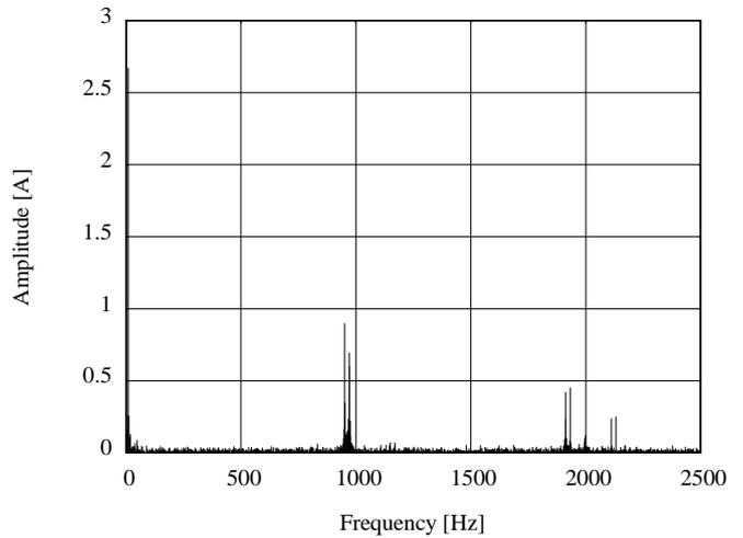
**Fig. 5.** Motor current spectrum at  $f_p = 10$  Hz
