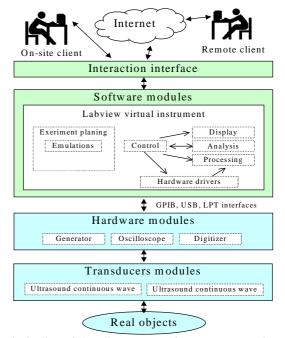
Fig. 1. Outline of the client – server internet connected remote experimentation system
