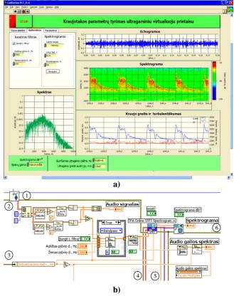
**Fig. 4.** Advanced ultrasound Doppler signal processing system: (a) - screenschoot of user interface, (b) - fragment of the algorithm diagram of the virtual instrument (1 and 6 - error messages, 2 – audio signal read from sound card, 3 – audio signal sampling frequency, 4 – setup parameters for time- frequency transformation, 5 – data output after time- frequency transformation)
