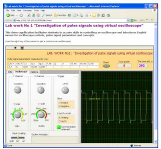
Fig. 2. The WEB based lab work which integrates three functional blocks: signal generator, oscilloscope and automatic "assessment"
