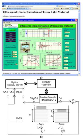
Fig. 3. Remote experimentation system: a - screenshoot of remote client user interface, b - structure of harware modules and real object
