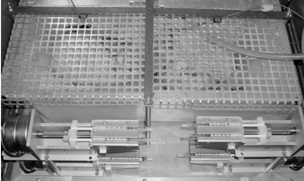
Fig. 4. Interior of a centrifuge cabin for testing of two experimental rats with a blood-withdrawing device
