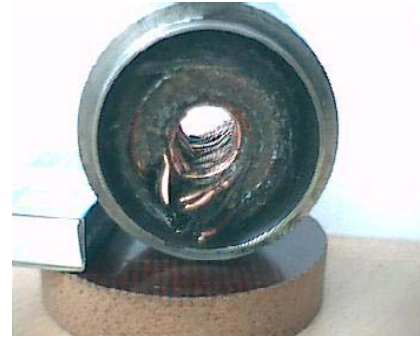
Fig.8. Destroyed pulsed solenoid
