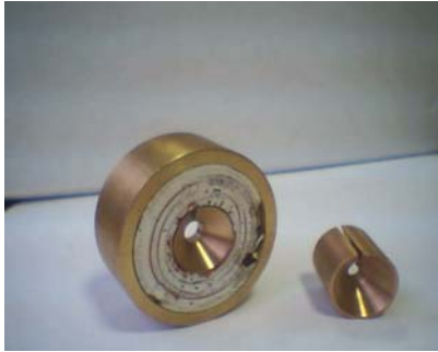
Fig.4. Pulsed transformer and flux concentrator
