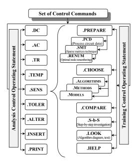
**Fig. 2.** Example of the set of control statements in the circuit design training system "Micro-PC"
