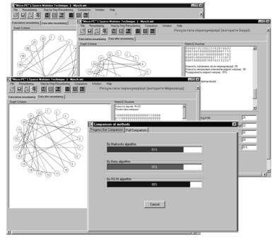
Fig. 3. Choosing and evaluation of different algorithms for optimal node renumbering
