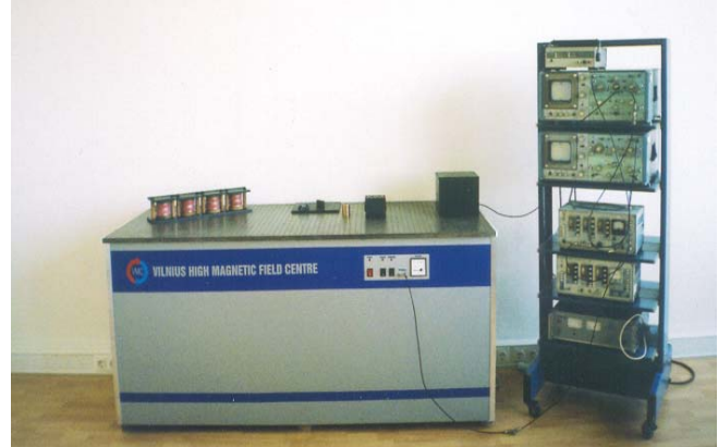
Fig. 6. Pulsed magnetic field generator up to 50 T with control and data registration devices
