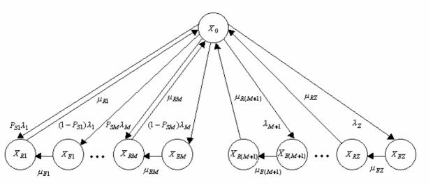
Fig. 1. Graph of change of states of the electronic device in exploitation at failures of components
