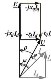
Fig. 9. Completed phasor diagram for the salient pole synchronous machine
