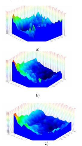
**Fig. 4.** Speech intelligibility in the classroom: a) sound source voice of lecturer; b) loudspeakers system 5.1; c) loudspeakers system 7.1
