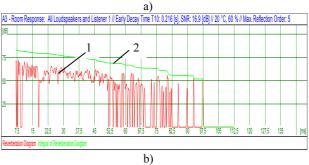
Fig. 7. Reverberation properties of classroom: a) ) sound source voice of lecturer; b) loudspeakers system 7.1. Where 1- reverberation diagram, 2- integral of reverberation diagram
