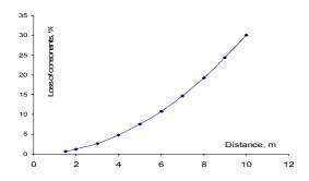
Fig. 8. The articulation loss of consonants
