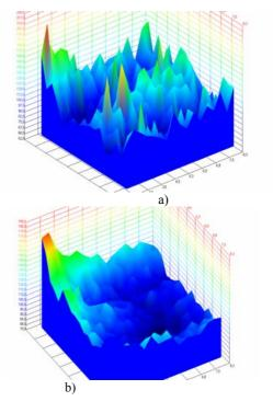
**Fig. 2.** Sound pressure level: a) sound source voice of lecturer; b) loudspeakers system 7.1
